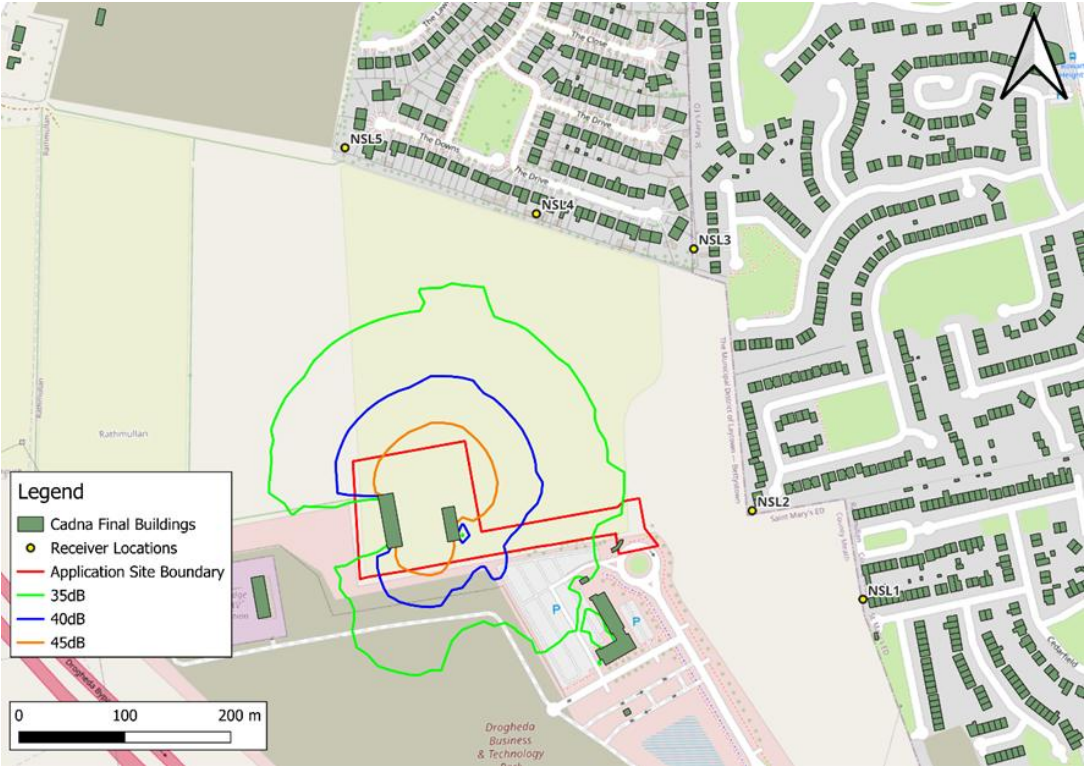
Figure 7.5: Noise Contours Plot of Predicted Operation Noise Levels for Scenario 2
